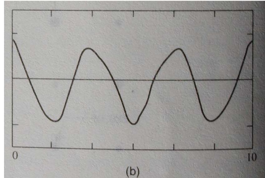
(b) The sampled cosine interpolated with a Gaussian display spot
