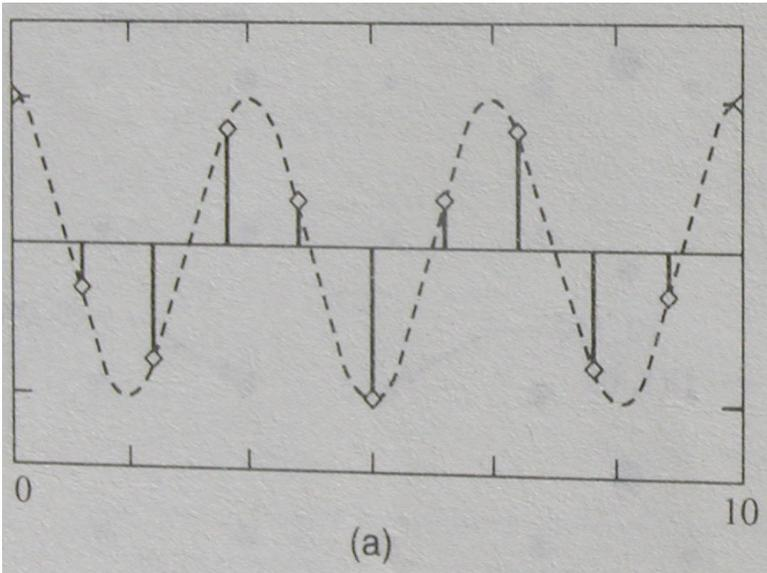
(a) The cosine sample at 3.3 sample per cycle
